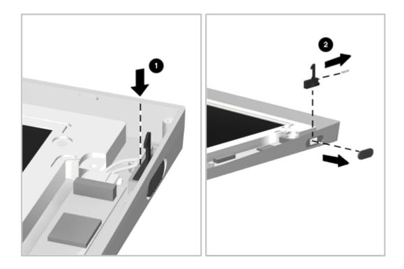
Figure 5-33. Removing the Latch Assembly
